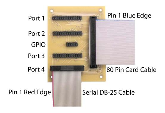
GND (1) (2) Port 3 IOA Port 1 IOA (3) (4) Port 3 IOB Port 1 IOB (5) (6) Port 4 IOA Port 2 IOA (7) (8) Port 4 IOB Port 2 IOB (9) (10) VCC
